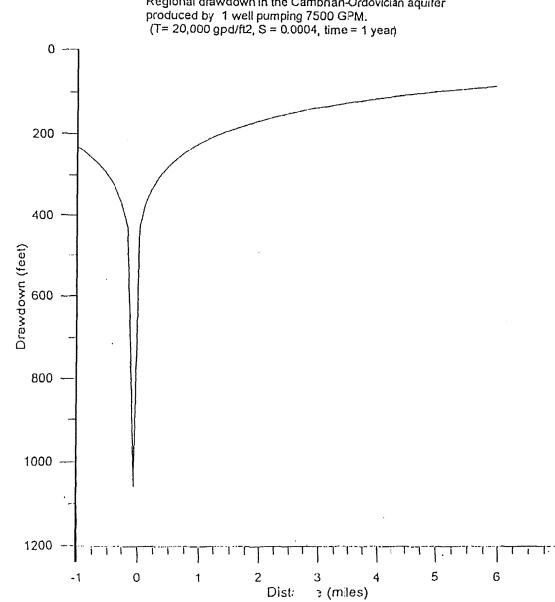
Regional drawdown in the Cambrian-Ordovician aquifer produced by 1 well pumping 7500 GPM. (T= 20,000 gpd/ft2, S = 0.0004, time = 1 year)
