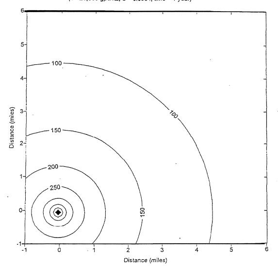
Regional drawdown in the Cambrian-Ordovician aquifer produced by 1 well pumping 7500 GPM. (T= 20,000 gpd/ft2, S = 0.0004, time = 1 year)
